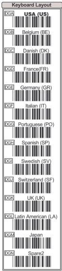
The selecting of keyboard layout supports many country languages other than USA keyboard layout. First you need to confirm country langage that you desire. In DOS, using command "Keyb" to selecte the desirable keyboard layout or in WINDOWS entry "Control" then pop "Keyboard" to selecte country at "language" item. For details, please refer to your DOS or WINDOWS user's manual.
