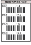
The setting is applied two kinds of ratio barcode symbologies with narrow and wide only, such as Code-39, Interleaved 2 of 5, Codabar, Plessey and IATA...etc. So, it will be ignored if some kinds of barcode symbologies, such as EAN, UPC, and Code-128, are read. This setting is able to adjust appropriate signal width during transmitting the bar image. The ratio allows to adjust from 12 to 13.5 but upon your wand decoder device.
