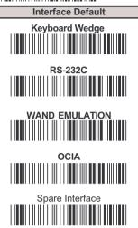
You can change factory interface default for other type interface. By plug different cable, program scanner and set right interface to exit, then the scanner will be change to another interface. However. you must make sure what cable vou need. Refer Cable Type to □ 66, 67.
