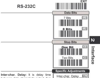
Inter-char. Delay: It is delay time between data character's output. It is same as <a href="Inter-char. Delay">Inter-char. Delay</a> of keyboard wedge, see <a href="12">12</a>.
